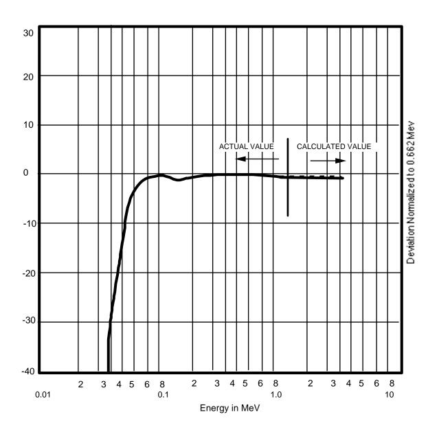
Figure 1-1. Detector Energy Response
