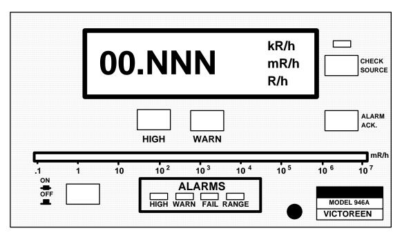
Figure 1-2. Front Panel, Model 946A-200 Universal Digital Ratemeter
