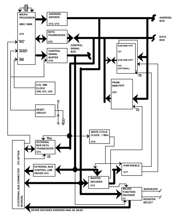
Figure 4-2. Page 1 of 3. Block Diagram - Main Circuit Board
