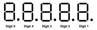
Data inputs D0-D3 and the decimal point, supplied by U72, are used to enter data in the selected digit as shown in Table 4-18.
