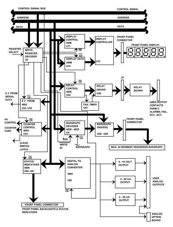
Figure 4-2. Page 2 of 3. Block Diagram - Main Circuit Board
