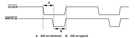
Figure 4-4. Write Cycle Clock Timing Diagram
