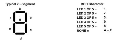
Assume that all bargraph segments are off. Example: Write hex data 38 to bargraph address 4020. Data 38 is stored, low byte (8) in U55 and high byte (3) in U56. Data (8) in U55 causes the code for an 8 to be output, which drives all output segments. The result is that the first five green LEDs turn on. Data (3) in U56 causes the code for a 3 to drive segments 1,2, and 3 connected to that device. The result is that the first 3 of 5 segments associated with U56 will turn on green.
