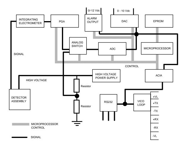
Figure 4-1. Detector Electronics Block Diagram
